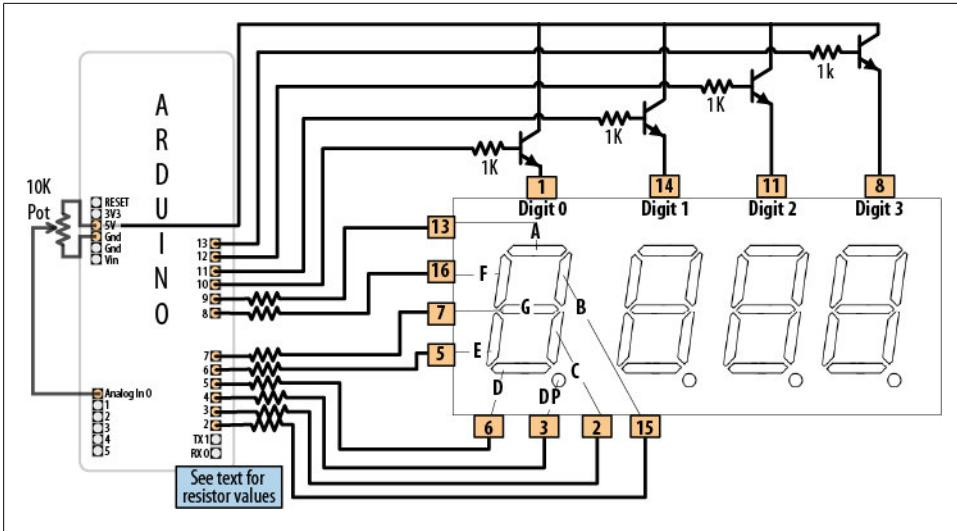
Figure 7-11. Connecting a multidigit, 7-segment display (LTC-2623)
