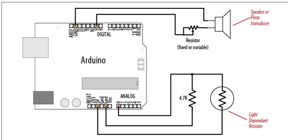
Figure 1-8. Connections for a speaker with the LDR circuit
